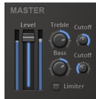
The **treble** knob controls amplification or attenuation of high frequencies. High values will amplify high frequencies and low values will dampen them. The **cutoff** knob paired with the treble knob controls at what frequency the treble knob starts affecting the sound.
